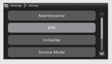
1 Select [DTC], and then press the ENT switch.
