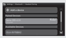
3. Select [Designate as a Rider] or [Connect Headset], and then press the ENT switch to [ON] (enable) the function.
