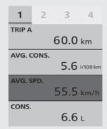
To reset the tripmeter A average speed [AVG. SPD.]: → P.64
