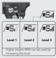
The selected level is maintained even when the ignition switch is turned to the (Off) position, or transmission is switched to out of S mode.
