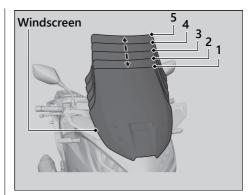
Check the windscreen adjustment for smooth operation and check the sliding area for looseness.
