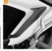
A set of two brushed aluminium-look fairing accents that mount directly to the existing fairing body. Easily installed and matches the 45L Top Box (Alu), 29L Pannier Kit, Panel Set (Alu), Leg Deflector Kit and Foot Deflector Kit.
