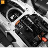
**U-Lock** Keep your Crosstourer safe with this tamper-resistant barrel key U-Lock that fits neatly under the seat.
