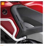
4 **Fairing Deflector Set** A set of left and right black polyurethane deflectors that fit to the upper and lower fairing and extend the amount of wind protection for both rider and pillion.
