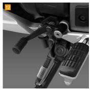
**DCT Foot Shifter Kit** A complete kit to select gears with a traditional foot shifter on the Crosstourer Dual Clutch Transmission model. Works in conjunction with, or in place of, the DCT handlebar shift triggers to offer a choice of gear selection styles.
