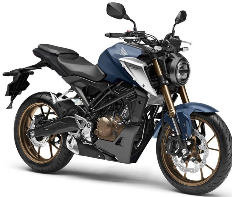
Model updates: Honda's premium Neo Sports Café 125 gets a power and torque boost from an all-new DOHC 4V engine, improving performance across the board. It also receives a major suspension upgrade – high-quality 41mm Showa's 'Separate Function' Big Piston (SFF-BP) USD forks, the first 125cc motorcycle in the world to do so.
