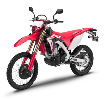
New model updates: Using the CRF450R moto-crosser as a base, Honda's new road-legal dual-purpose motorcycle has a tough, lightweight chassis built to find all the available grip, powered by an engine that delivers strong, usable power right from the bottom. Durable, high quality parts and long service intervals aim for a worry-free riding and ownership experience.
